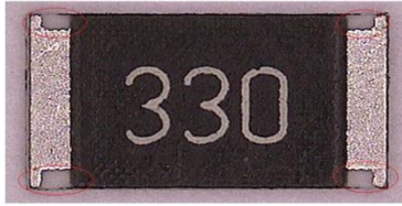
Pic 10 Electrodes after electroplating
