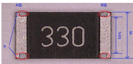
Pic 11 image of the electrodes after electroplating
