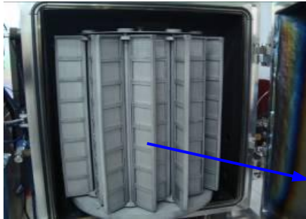
Pic.5 Vacuum sputtering chamber
